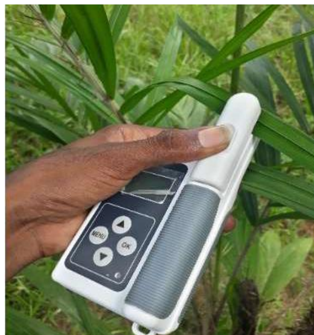
Figure 6. Obtaining leaf greenness values using the chlorophyll meter.
